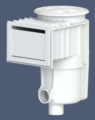
QuikSkim is a vital part of your cleaning and circulation system. With its venturipowered skimming, natural water pressure creates a stronger vacuum to clear more debris than a standard skimmer.
